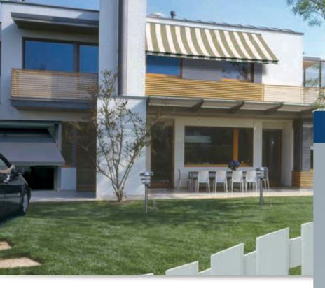
Bannette<sup>™</sup> Awnings come in two configurations - with or without arms. The Drop Arm version is ideal for small windows and balcony applications for internal shade and sun protection. The factory assembled arms are sprung to provide even tension on the fabric and are controlled by a gearbox and crank handle or motorised.
